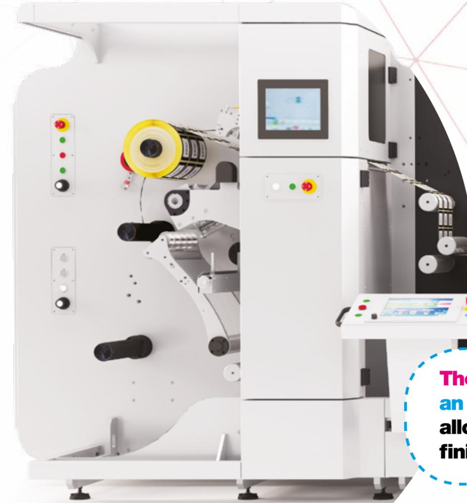
**The AutoSet is also available as an option on the Digicon Series 3, allowing digitally printed labels to be finished completely in one process.**
